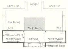
Elevator minimum area 50% of stage. Each vault maximum area 150% of elevator
