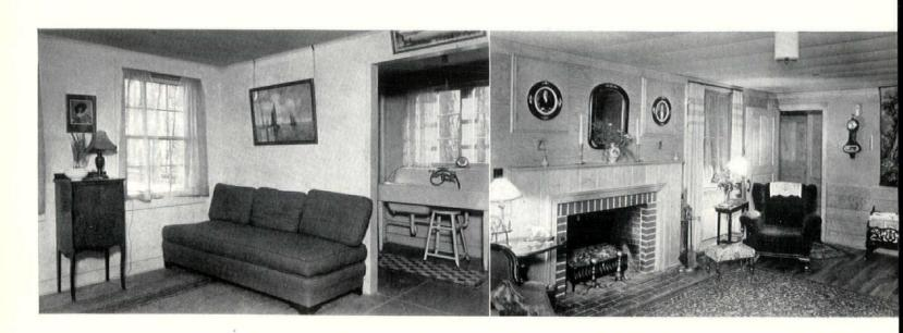
(Above) Painted cinder block for interior walls and the warm browns and reds of the precast floor have proven both economical and satisfactory. (Right) The walls of living room have horizontal pine ship lap below the dado and plywood above
