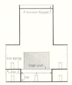
Two ducts through wall are permitted below stage if of 3 hr. fire resistance rating construction for 10 feet each side of wall. (Not
