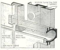
Typical Pointed-Joint Construction. Reproduced 1/2 Full Size
