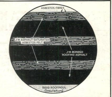
Enlarged Roofing Cross-Section Shows Why J-M Asbestos Felts Protect the Waterproofing Asphalts from the Sun
