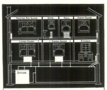
This shows you how simple the Burnham Unit-Air Conditioner System is. The Unit-Air Conditioners are located in the living and dining rooms downstairs and the master bedroom upstairs. Rest of heating done by the Burnham Slenderized Radiators.
