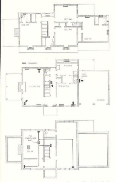
Figure 3. Layout for an Auxiliary System in the same plan as that used for the other two systems
