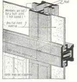
Typical Capped-Joint Construction. Reproduced 1/2 Full Size
