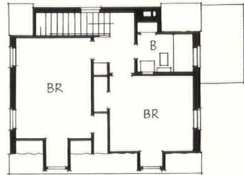
At right, first and second floor plans of a type of single family dwelling. To compensate for lack of cellar storage space, a hatch is provided in second floor ceiling, giving access to attic space
