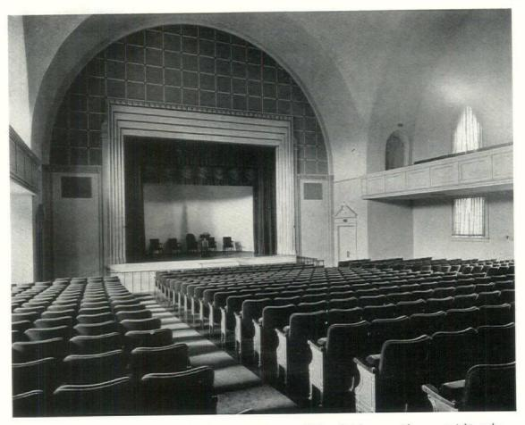
Typical three-bank auditorium seating laid out in straight rows. Notice that because aisles are at right angles to seats rows end seats do not project. Seats at fronts of side-banks and balconies will not provide good vision but as this is obviously an auditorium rather than a theater, such a defect may be tolerated
