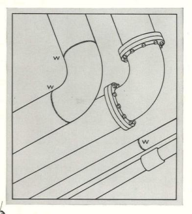
The welds, "W", are smooth inside and flush with the pipe wall on the outside. Each weld is inherently more simple than any other joint can possibly be.
