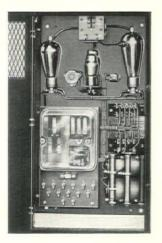
Ward Leonard Electric Co., Mount Vernon, N. Y. has developed two automatic electronic alternator voltage regulators. They have no moving parts. Instead of relying upon mechanical means to close contacts or change pressures an inertialess stream of electrons controls the regulating action. These regulators are controlled rectifiers deriving their power from the a.c. generator and delivering the rectified d.c. current to the shunt field of the exciter in an amount which is a function of
