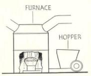
STOKER-FIRED FURNACE WITH HOPPER FEED
