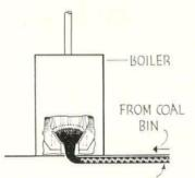
FEED MECHANISM (MOTOR DRIVEN) STOKER-FIRED BOILER WITH FEED FROM BIN
