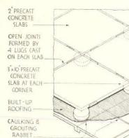
PRECAST CONCRETE STRUCTURAL SLABS
