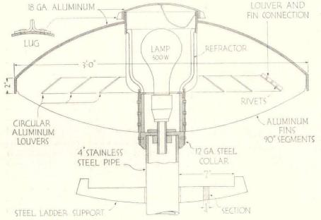
This hooded fixture was designed for the illumination of parking spaces in the vicinity of the dam, where spill of light beyond the area to be lighted is objectionable. The hood and louvers cut off direct view of the refractor beyond that area. Light distribution within those limits may be controlled by the choice of the refractor and by adjustment of the bulb center. The fixture may be relamped from the top
