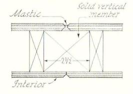
Figure I (left). Section showing typical assembly of floor, wall and roof panels. Figure 2 (above). Plan showing solid vertical member fitted into the grooves on the sides of adjacent wall panels
