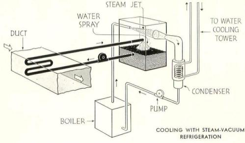
**Steam - Vacuum Refrigeration** has only recently come within the field of normal architectural practice, having hitherto been adapted to relatively large installations requiring special engineering design. Today steam-jet refrigerating units are available in sizes small enough for use in the larger residences or equivalent store, restaurant or commercial and institutional structures.
