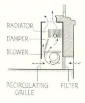
UNIT VENTILATOR WITH HEATER AND FORCED CIRCULATION
