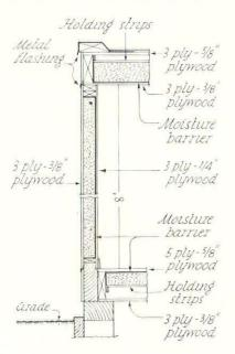
lar to that for the interior wall surfaces but is slightly opened, and the inside is beveled to form a pocket for mastic which is placed between the panels directly after erection. This pocket permits a sufficient amount of mastic to be placed between the panels so that it will remain plastic indefinitely, and thereby make a tight and permanent seal against the entrance of moisture and infiltration of air through the exterior panel joints.
