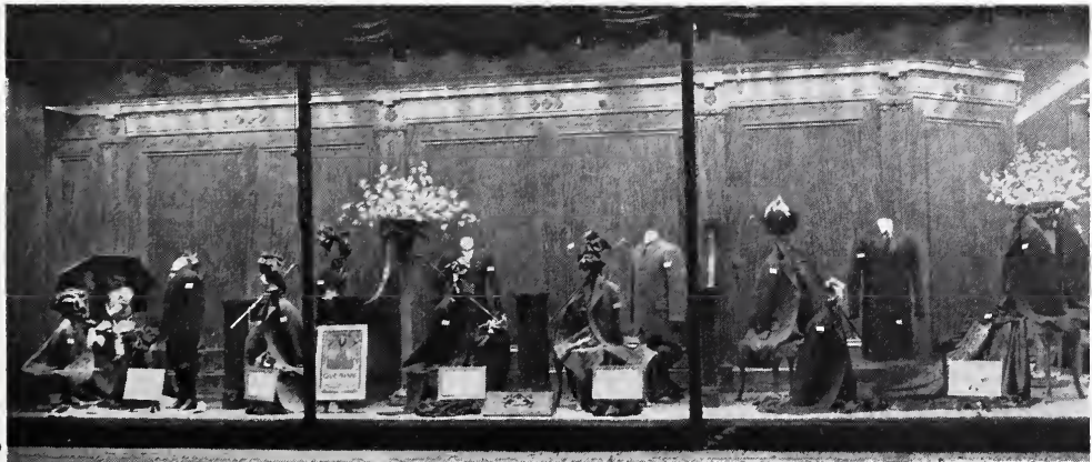
FIG. 4. POLISHED WOODWORK CAUSES GLARE AND REVEALS THE LOCATION OF LAMPS AND REFLECTORS.
