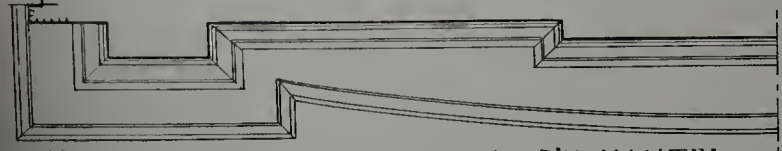
1/2 PLAN OF SHELF OF DINING R'M. MANTEL LOOKING UP - LIVING R'M. MANTEL SIMILAR
