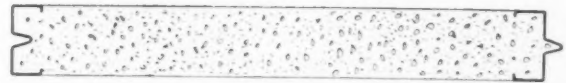
Cross section through Gypsum plank, showing tongued-and-grooved steel edges and ends, forming continuous I-beam entire length of plank.
