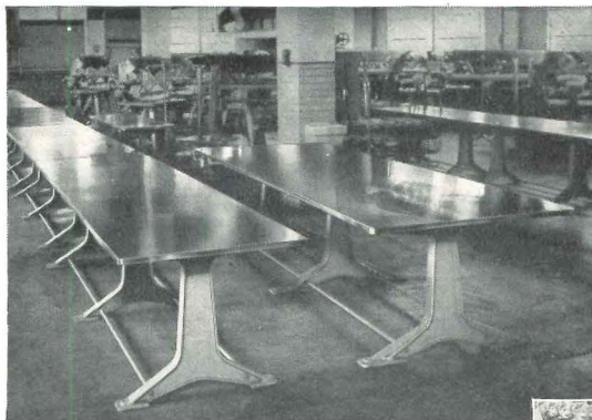
(Left) 10 of the 18 Smith-Drum Monel Tables installed in same laundry: thirteen 31" x 120"; four 50" x 120"; one 26" x 76".
