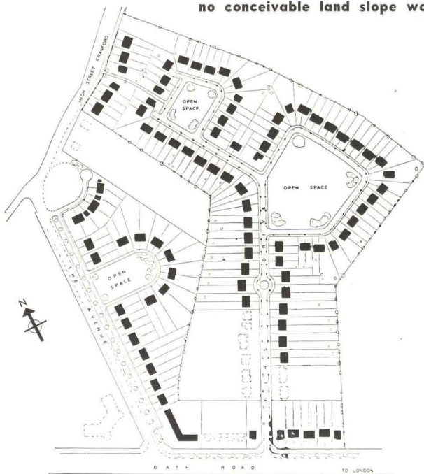
GRANFORD ESTATE. For this estate the Laing architects prepared several layouts and found it meant either a very dense development or an open one as shown. This open development resulted in such an attractive scheme that the extra expenditure for roadways and land was considered fully justified.
