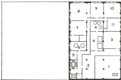
Plan, 11th floor: 1, air conditioning; 2, experimental brewery; 3, water cooler; 4, experi- mental cellar; 5, 6, yeast rooms; 7, 8, laboratories; 9, li- brary; 10, drafting; 11, superintendent.
