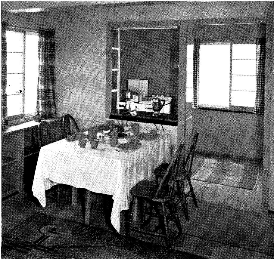
Dining space and kitchen of the experimental house. Dark strips at counter, at base of bookshelves, and at kitchen windowsill are a new type of electric service strip, prefabricated in standard lengths with integral plug-in outlets. Strip provides flexible electric service in every room.
