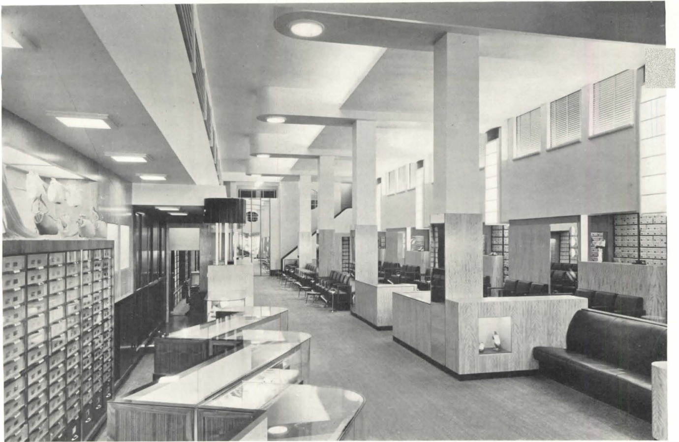
Interior from left of entrance: serrated hosiery counter in left foreground, enclosed catwalks on either side. View shows effect of concealed lighting in lip of lower plane of the two-level ceiling and in mezzanine window sills.
