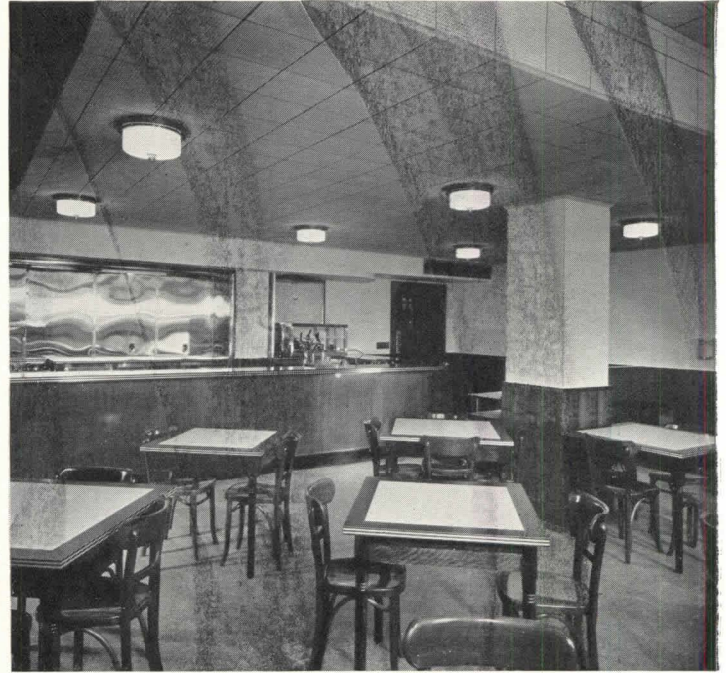
Coffee shop, or public dining space, in same hospital; note acoustic treatment of ceiling.
