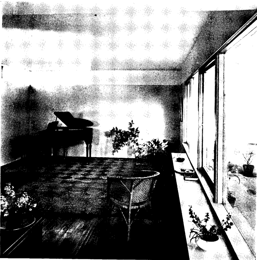
Toward the patio, the sill level of the windows is dropped to 26 in.
