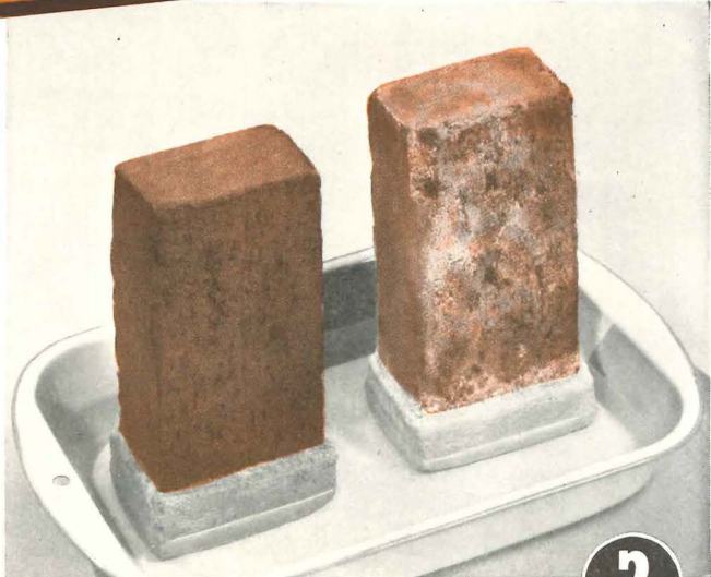
Keep about an inch of water in the pan. Even if soluble salts are present in the brick or sand, you will soon be convinced that Brixment mortar helps prevent efflorescence. (Photo 2.)
