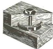
TECO Ring Connectors spread the load on a timber joint over practically the entire cross-section of the wood.
