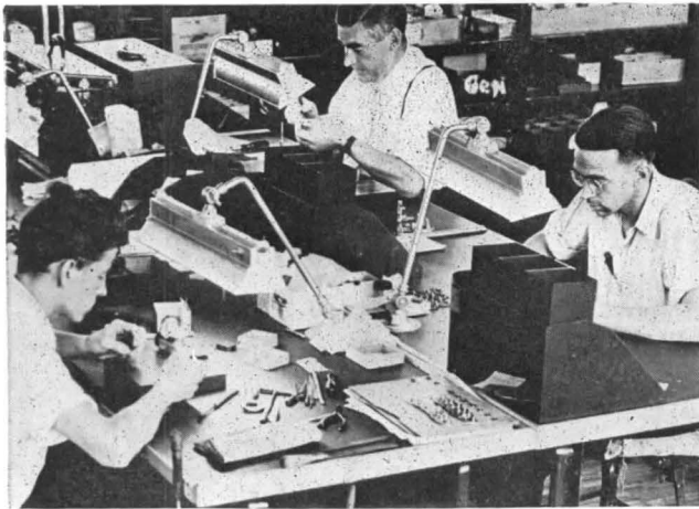
Older or defective eyes are enabled to function more efficiently and with less fatigue when assisted by good illumination properly located with respect to the work
