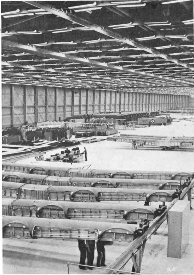
White floor acts as huge reflector and permits work to be performed under wings of planes without having to resort to auxiliary lighting on the assembly line of this great aircraft plant
