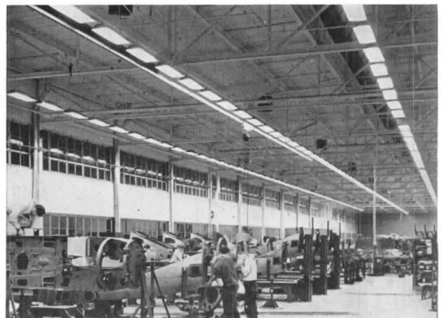
Fluorescent lamps in rows of individual fixtures give uniform lighting for the manufacture of fighter planes, with high intensity light and a minimum of shadows at the level of the work
