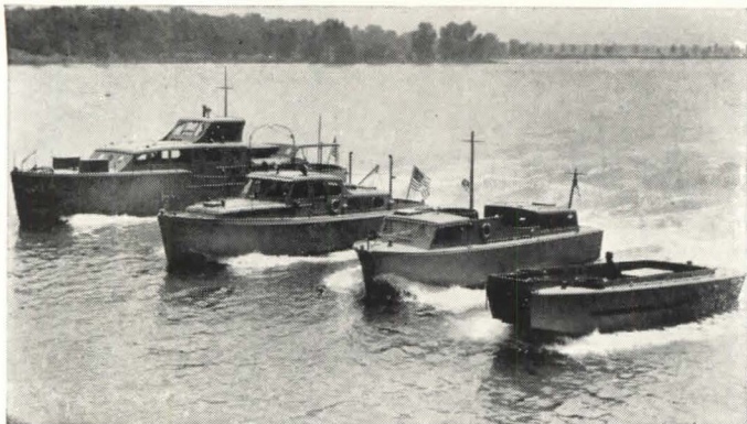
Four outstanding boats built by Chris-Craft with exterior-type fir plywood: (from left) U. S. Army Q boat, U. S. Army Aircraft Rescue boat, U. S. Navy Picket boat, U. S. Navy Troop Landing boat.
