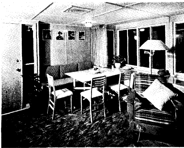
Built-in furniture and dinette set are of white pine in natural finish; other furniture in maple, commercial finish close to natural. Plywood floor covered with marbled linoleum in blue
