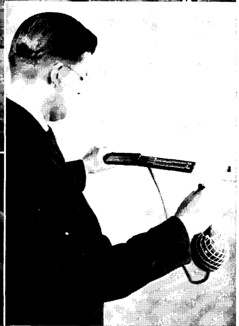
Taking Humidity Readings with Hand- Aspirated Psychrometer.
