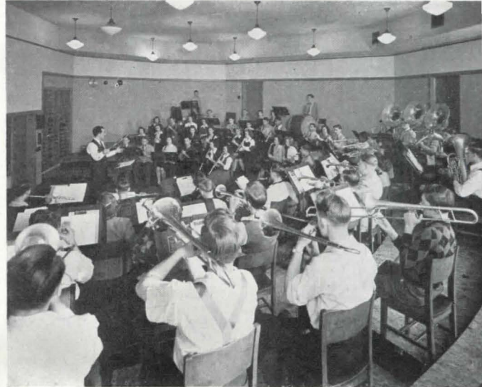
Band rehearsal room has high-coefficient acoustic ceiling. The adjoining room, for vocal work, has much less correction. Instrument storage space separates the two rooms
