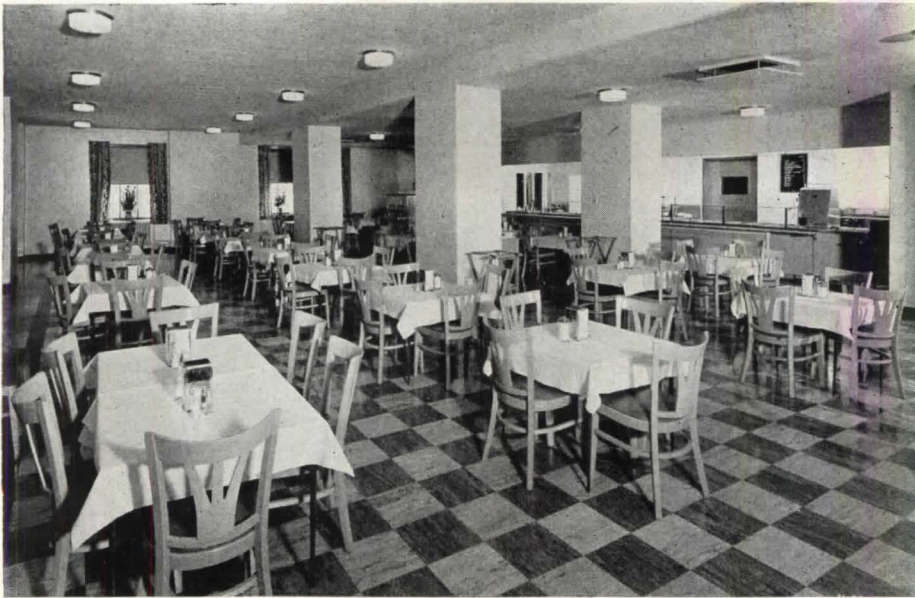
Nurses' cafeteria (see second floor plan) has acoustic tile ceiling, asphalt tile floor, mechanical ventilation system
