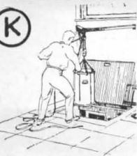
ASH REMOVAL BY USE OF REMOVABLE BRACKET & TACKLE
