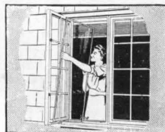
DUAL GLAZING —a single panel type that mounts on inside of sash. Inconspicuous. Easily removed for cleaning.
