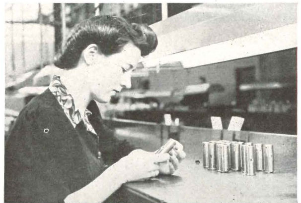
14-15. With good supplemental lighting the worker can either utilize or avoid specular reflections from polished objects. White background increases visibility
