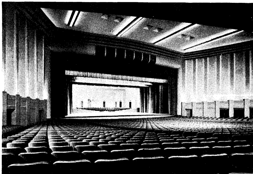
Fig. 10: An RCA listening studio: good sound distribution with convex panels
