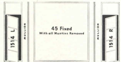
Remove all muntins from Ceco stock casement 45-Fixed. Combine windows with standard mullions.
