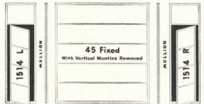
Remove vertical muntins from Ceco stock casement 45-Fixed. Combine windows with standard mullions.
