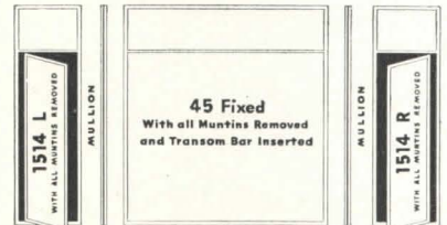
Remove all muntins and insert transom bar as illustrated. Combine windows with standard mullions.
