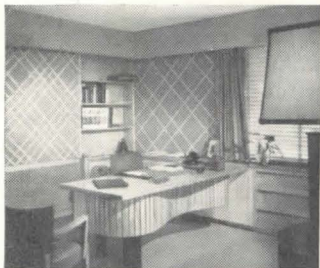
OFFICES. Birch Weldwood combined with wallpaper. Valance is decorative and practical — it conceals drape and blind attachments, and provides space for indirect lighting fixtures at the same time.
