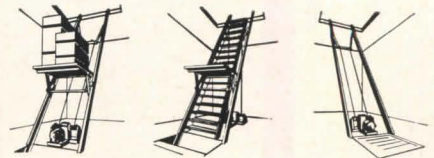
Stairlevayor, a motorized lift designed for use in open spaces or over stairways
