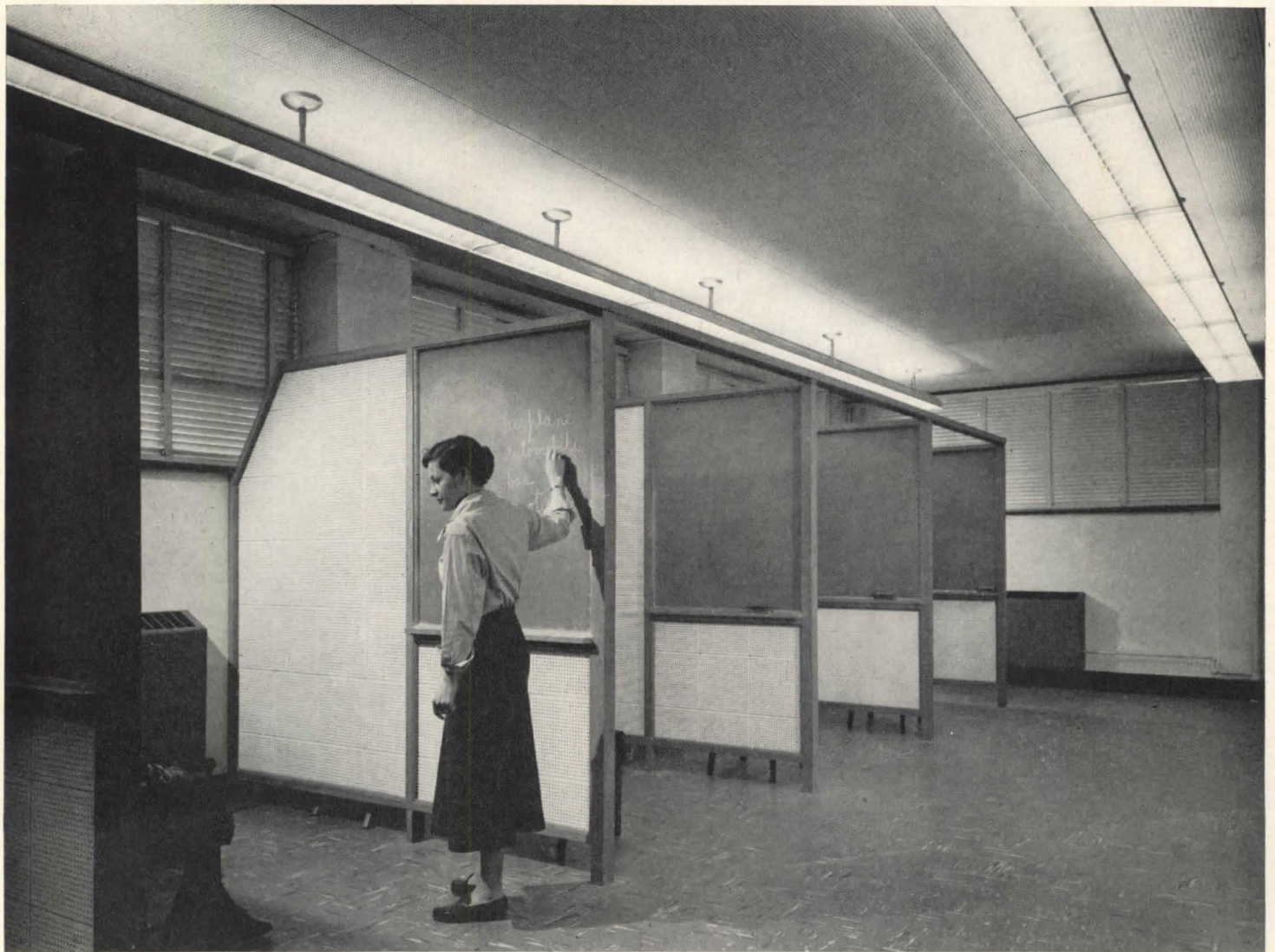
Top: rooms used by public, pupils or patients are furnished as pleasantly as possible. Throughout, floors are asphalt tile and ceilings acoustical tile. Below, speech clinic contains cubicles large enough for teacher, pupil and a parent or friend to help put pupil at ease
