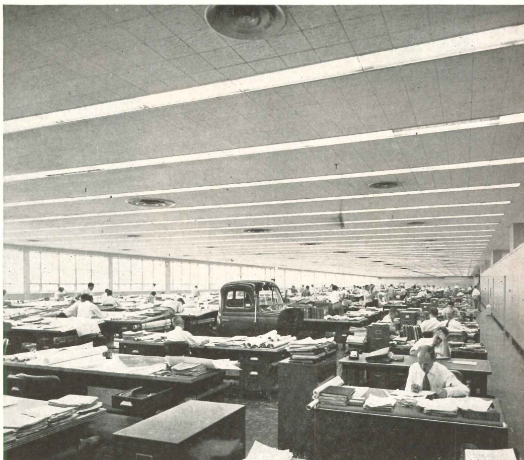
Drafting room is 420 ft long, 100 ft wide. Overhead lighting, giving 70 foot-candles, was carefully designed to prevent excessive brightness when the eye looks lengthwise of room
