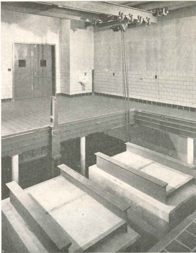
In the dynamometer test wing all sorts of strange operations go forward. Above, "typical double end engine development test cell." Right: an engine under test, driving generator; incidentally, generators feed into electrical system, and so put to use power of engines under test. Below: main corridor in dynamometer test wing
