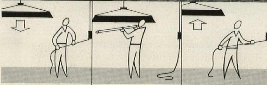
A Only a detachable handline is required to disconnect and lower a luminaire.
