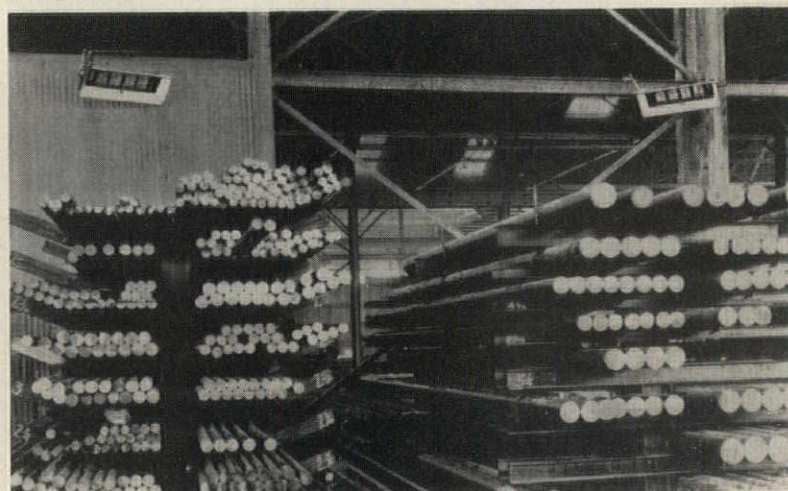
Angle-mounted generators check condensation on steel stocks; keep temperature minimum 10 F above dew point
