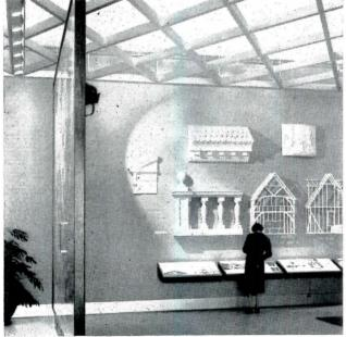
Diffuse lighting gives the low contrast illumination necessary for prolonged visual tasks, but it well nigh obliterates the highlights, shades and shadows by which we perceive form and texture. By introducing some variation in brightness, the monotony of such a space can be relieved, and the form and texture of included objects re-emphasized at no expense to the observer's ability to study them
