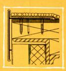
Typical detail and photo of Kaiser Aluminum's Type K-1 Gravel Stop.
