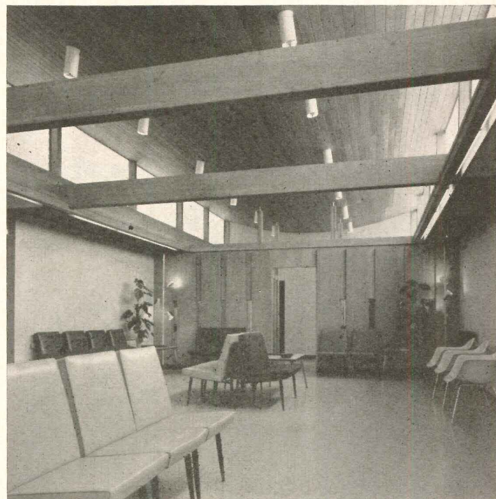
The central waiting room is located for efficient handling of patients bound for various departments. A pleasant feeling is achieved by the use of clerestory windows, exposed beams, and the reverse-curve roof
