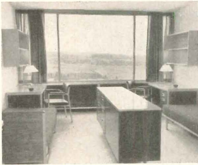
Typical two-man living unit, 18 ft 6 in. by 13 ft 4 in., has sliding aluminum windows, walnut wardrobe and storage units, double lavatory, sand-finish plaster walls
