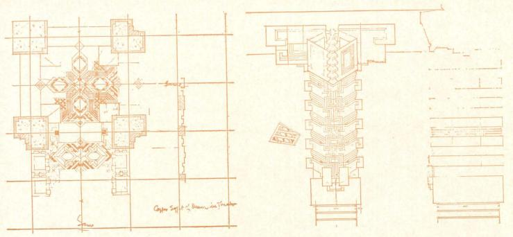
Pencil studies by Wright. At left, copper soffit of beam in theater, at right, a pier cap
