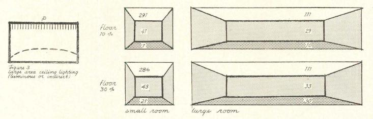
With large ceiling lighting systems the ceiling itself is the primary source and its brightness is relatively high. Walls and floor are secondary sources which correspond to those produced by general diffuse lighting, and have about the same relative brightnesses. The illumination level is more uniform than with either of the other two basic light systems
