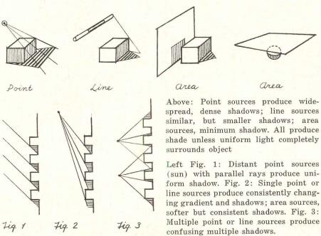
very little since the included angle is little changed. On the other hand, when the included angle is small, as in a small or high room, the ceiling may have to be twice as bright to produce equivalent illumination. Using the walls as additional sources, however, can increase the solid angle so that the required illumination level can be achieved with a lower brightness source.
