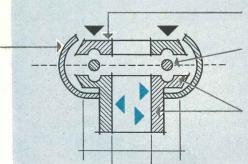
Case hardened steel top raceway. Knuckle rides on this.
