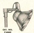
New Aluminum Enclosed Angle Type Floodlights-Alzak Finish, Wide or Narrow Beam-for Incandescent 750-1500 Watt Lamps or Mercury Vapor 400 Watt Lamp.
