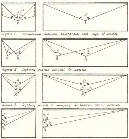
Figure 4 lighting planes perpendicular to source
