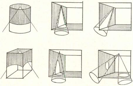
Since distribution from point sources is essentially conical in spite of fixture variations, light patterns necessarily will correspond to those produced by a cone of light
