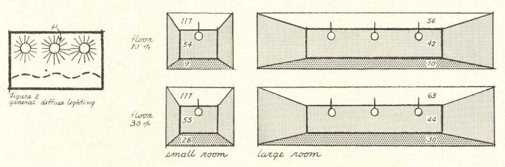
General diffuse systems throw direct light to all surfaces so that relative brightnesses are affected primarily by surface reflectances. All surfaces act as secondary sources with the walls assuming particular importance, especially in small rooms. Note that the gradient, though still non-uniform, is less "bumpy" than that of down lights.
