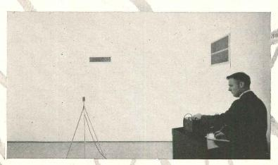
enough to assure comfortable environment, for sound must be measured and specified not only in terms of over-all magnitude, but also in magnitude at different frequency levels.
