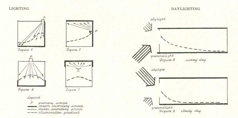
reflectances are higher than 50 per cent, particularly in small rooms; the walls can in fact assume major importance as supplementary light sources. Conversely, dark-colored walls would absorb a large portion of the light supplied by the fixtures.
