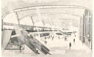
Arvin Shaw III, Carson & Lundin: 2-story concourse is daylighted by large glass areas in front and rear walls and skylights between barrel vaulted roof sections
