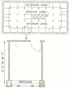
Figure 1: Typical block type building showing interior and exterior zones
