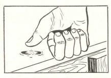
5. Give final steel troweling when thumb pressure barely dents the concrete surface.
