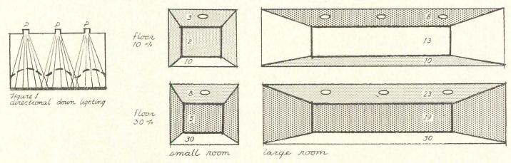
With directional downlighting, ceiling, which receives no direct light from fixtures must be darker than floor regardless of floor reflectance. However, lighter floors increase effectiveness of walls as secondary sources, thus brightening ceiling and helping to level out sharp curves shown as characteristic of illumination gradient on horizontal work plane
