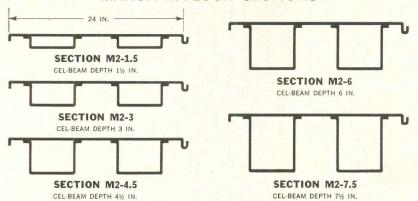
Note: These M-Floor Sections are also available with cell elements having integral stiffening ribs for improved section properties.
