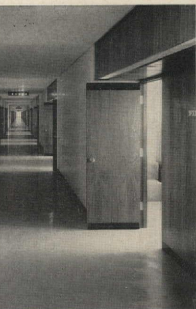
Above: Since principal lighting emphasizes shape of these structures, conflicting patterns from wall fixtures are minor blemishes. Far left: Downlights render circular surface neutrally, but change in pattern provides added contrast with surrounding ceiling. Left: Light sources designed to relate to door recesses rather than to deliver "X" footcandles define shape of corridor, aid orientation, provide enough light for circulation
