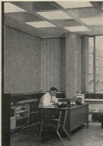
Above: Merely recessing lighting equipment into it does not necessarily define structure. Bands of light in schoolroom at right simply dominate the space; in office at left, enough modules are used for light control to help outline structure. Below: Light pattern from wall-mounted source, and shape of fixture itself, are appropriate to triangular walls. A similar pattern disorganizes rectangular wall at left
