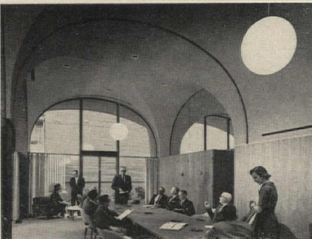
Above right: Structure can be accented by controlled reflectances (e.g., light beams against dark ceiling), or by planned brightness gradations. Below right: At night, bullets will throw confusing splotches of light on roof. Above: Globes are logical shapes, logically placed to light high vaulted ceiling and supplement daylighting
