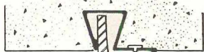
As a METAL WINDOW REGLET used at head only for single sash and at head and jambs for multiple frames.
