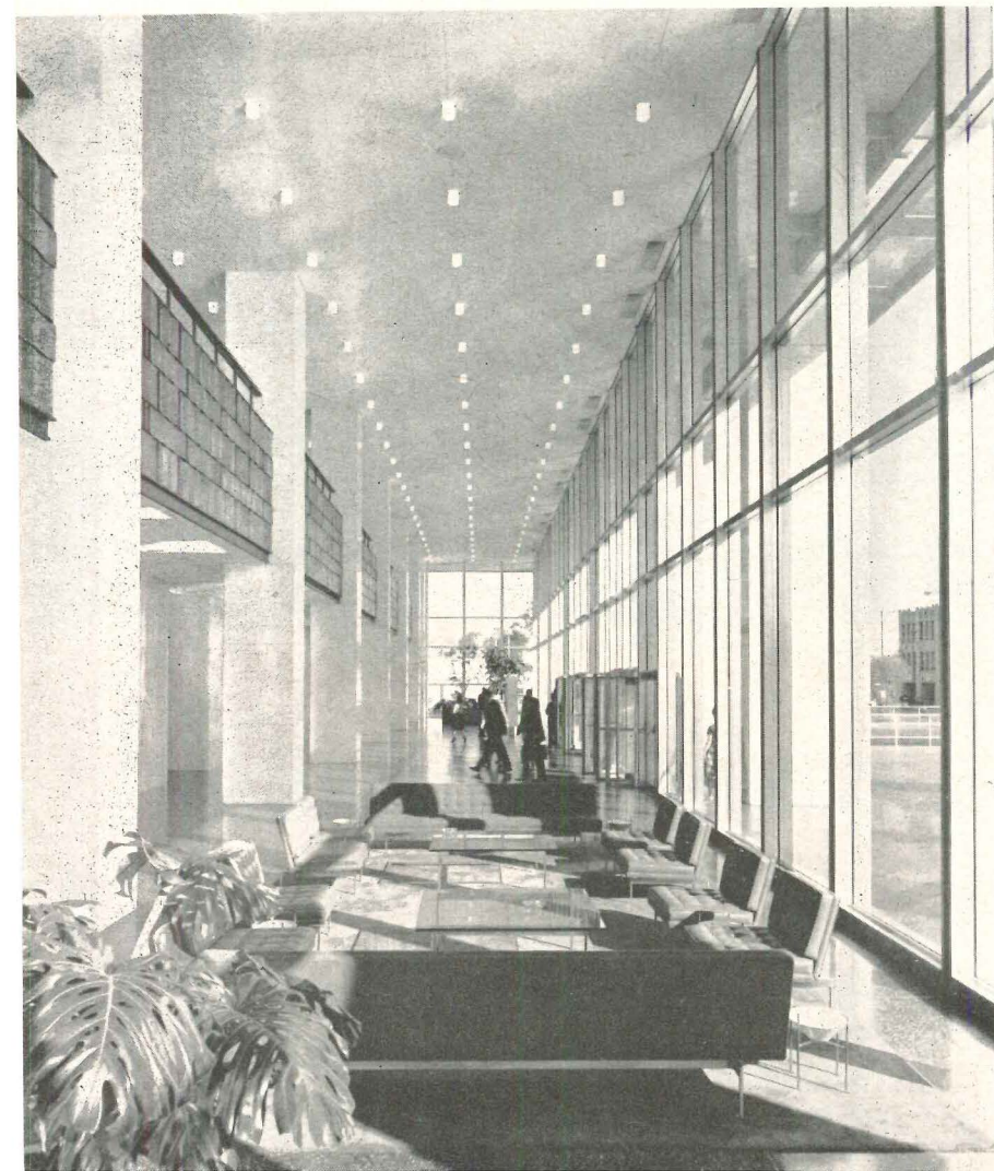
Above: Sun screen is composed of approximately 14,000 individual porcelain enameled aluminum panels. Below: North and south lobbies are 29 feet high. Mezzanine is faced with formed bronze pans, terrazzo floors are charcoal brown to match the exterior podium, chairs and sofas are burnt orange, carpets are gold, columns are finished in white Vermont marble, and the elevators are warm-toned travertine
