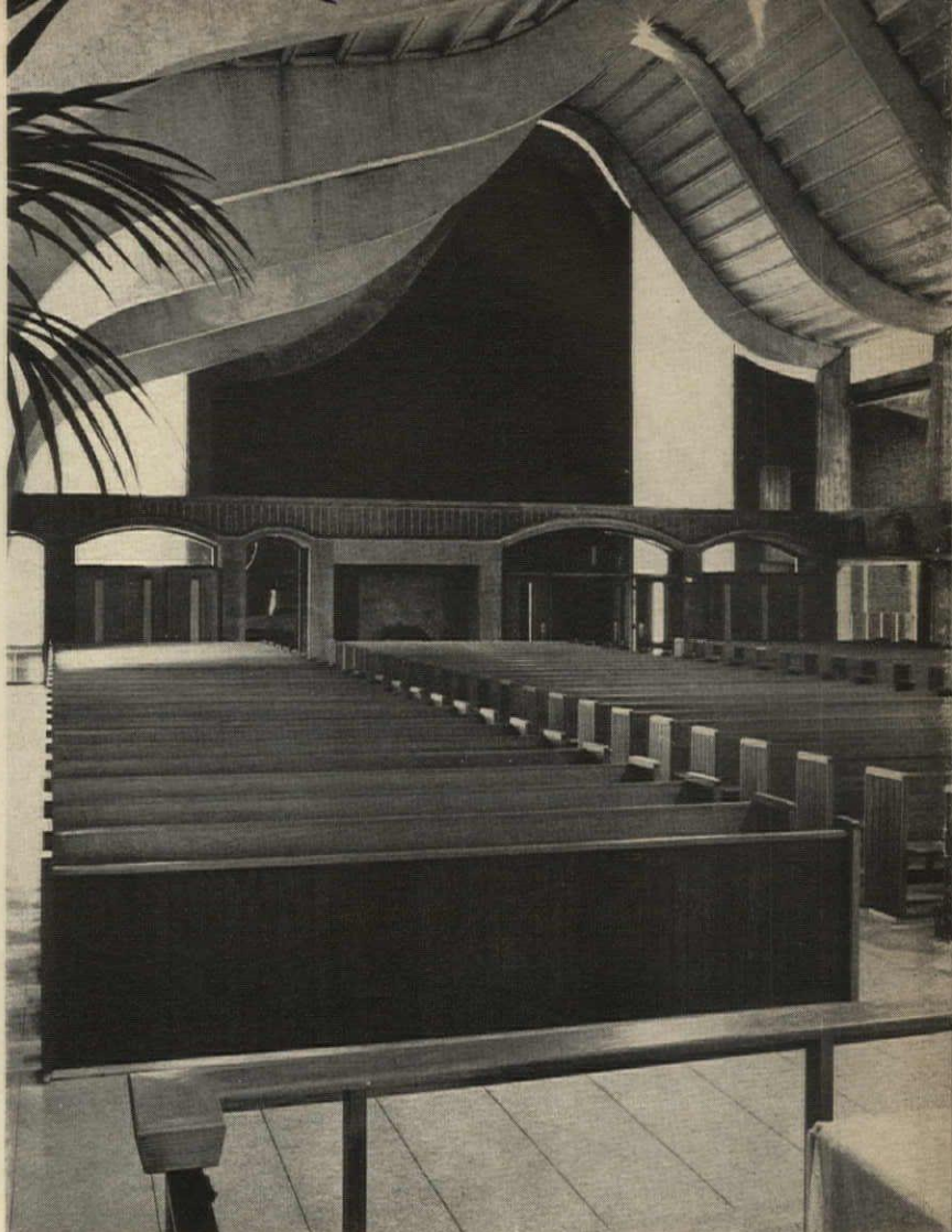
Walls are rough grey-buff brick. Translucent panels are fiber glass.
