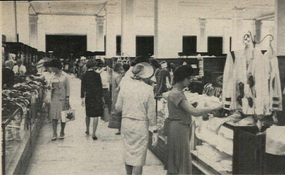
In this department store the high brightness of the ceiling and columns far exceeds the brightness of the merchandise, drawing the eye upwards away from the sales counters. Although the uplighting "enlarges" the space, downlighting should have been used with the uplighting to emphasize the sales counters.
