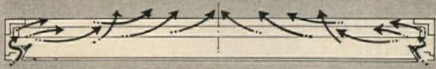
AIR FLOW PATTERN —Air moves through diffuser frame air controllers, passes over the lamps and ballasts, and out through slots in troffer center area.
