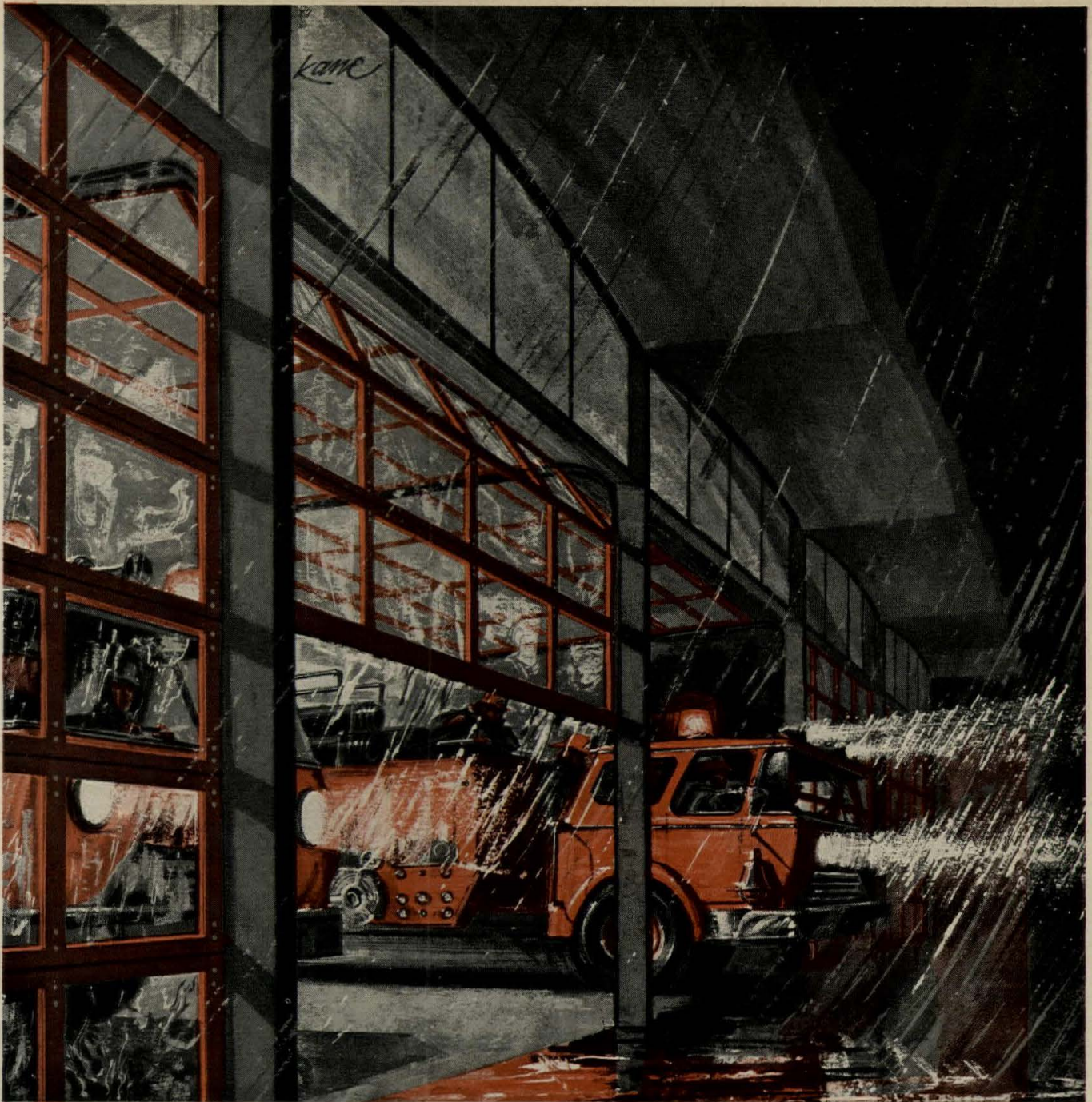
Central signal station automatically controls these fire station doors—closes them 90 seconds after signal sounds
