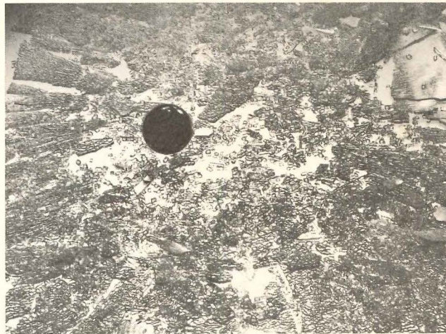
Tempered glass is stronger, more costly than common glass but disintegrates into tiny fragments when struck; still must be replaced.
