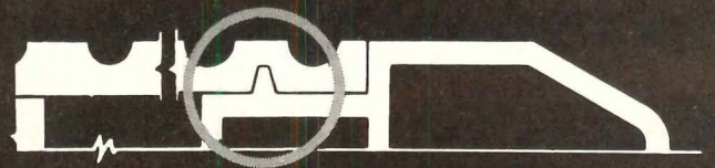
Saddle Assembly. Interlock between plate and support section eliminates drilling and tapping. Secure fit guaranteed. Easy installation.
