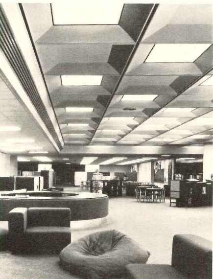
LIGHTING/CEILING SYSTEMS / The company offers distinct lighting/ceiling systems with replaceable and interchangeable modular suspension components. The "Vaulted Linear" (VL60), "Vaulted Directional" (VN60), and "Flat Linear" (FL60) are the same basic 5-ft sq ceiling planning module. Each module can be rotated 90 degrees and is designed to accommodate its own lighting, partitioning, acoustics, air distribution, sprinkler penetration and easy access. Unlighted modular choices are available. ■ Conwed Corp., St. Paul, Minn.
