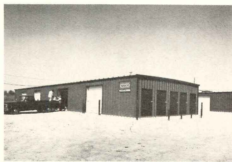
MINI WAREHOUSES / A building system for construction of mini warehouses is available in standard 5-ft width increments from 20 ft to 35 ft spans. The buildings feature metal roofing with ¼-in. per ft slope. Eave heights up to 16 ft are a standard feature and integrated wall panels are offered in various color options. ■ Butler Mfg. Co., Kansas City, Mo.
