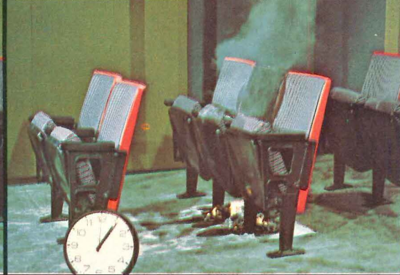
Major flames out. Time: 6 minutes, 00 seconds. Damage: 1 chair involved, fabric melting and smoldering on two adjoining chairs.
