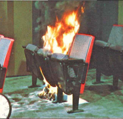
TEST ONE: DU PONT NEOPRENE Time: 1 minute, 30 seconds after ignition.
