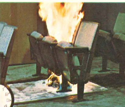
TEST THREE: STANDARD POLYURETHANE Time: 1 minute, 30 seconds after ignition.
