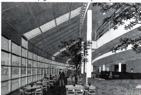
A long gallery gives relief to large open-plan areas and provides an interior street in AT&T's 400,000-sq-ft Long Lines Eastern Area Headquarters, Oakton, Virginia, designed by Kohn Pedersen Fox Associates, Architects. To meet energy-code requirements, reflective insulating glass was used throughout, and a large portion of the curvilinear cafeteria enclosure has opaque insulated panels. Insulating glass is heat-strengthened, and the inboard light is laminated. Skylight fabricator: Super Sky Products.
