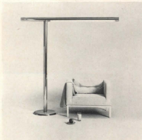
FLOOR LAMP / A 72-in long arm is cantilevered from a 72-in. high polished chrome stand. A clear linear prismatic acrylic diffuser runs the length of the illuminated opening; a 40 Watt fluorescent tube is recommended. ■ Habitat, New York City.
