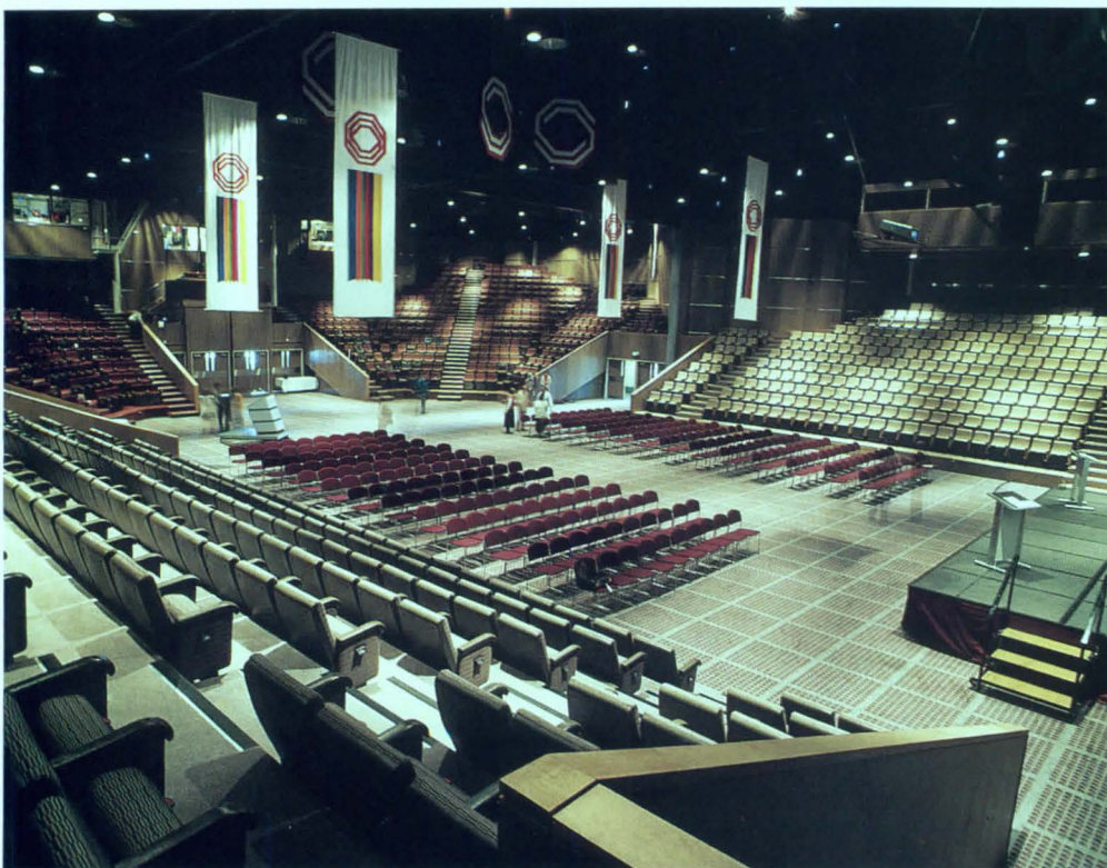
Oriented outward to a lakefront park (opposite) as well as inward to a plaza forecourt, Adelaide's center hosts a variety of events in a hall that can be converted from a 3,500-seat raked auditorium (left) to a flat-floored banquet/exhibit space (above) by raising the hinged seating platforms.
