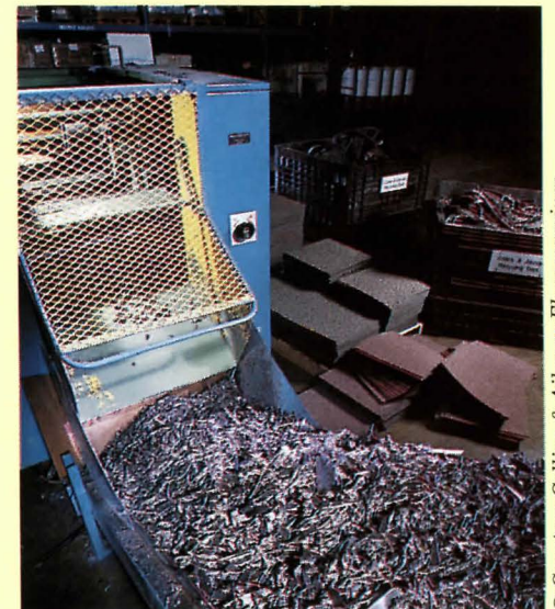
Vinyl-backed carpet and tile being shredded during recycling, en route to becoming highway sound barriers.
