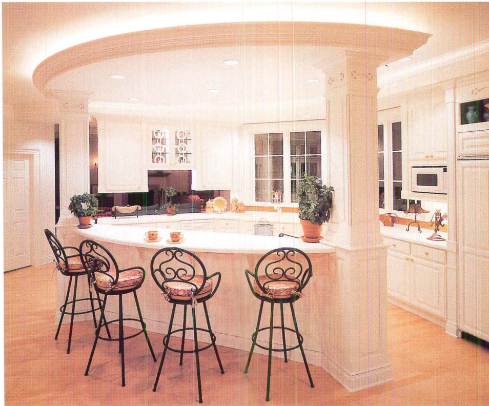
Black Alzak-cones in downlights (above) completely eliminate glare at the ceiling plane. A-19 lamps in open reflector downlights cover lots of horizontal space.
