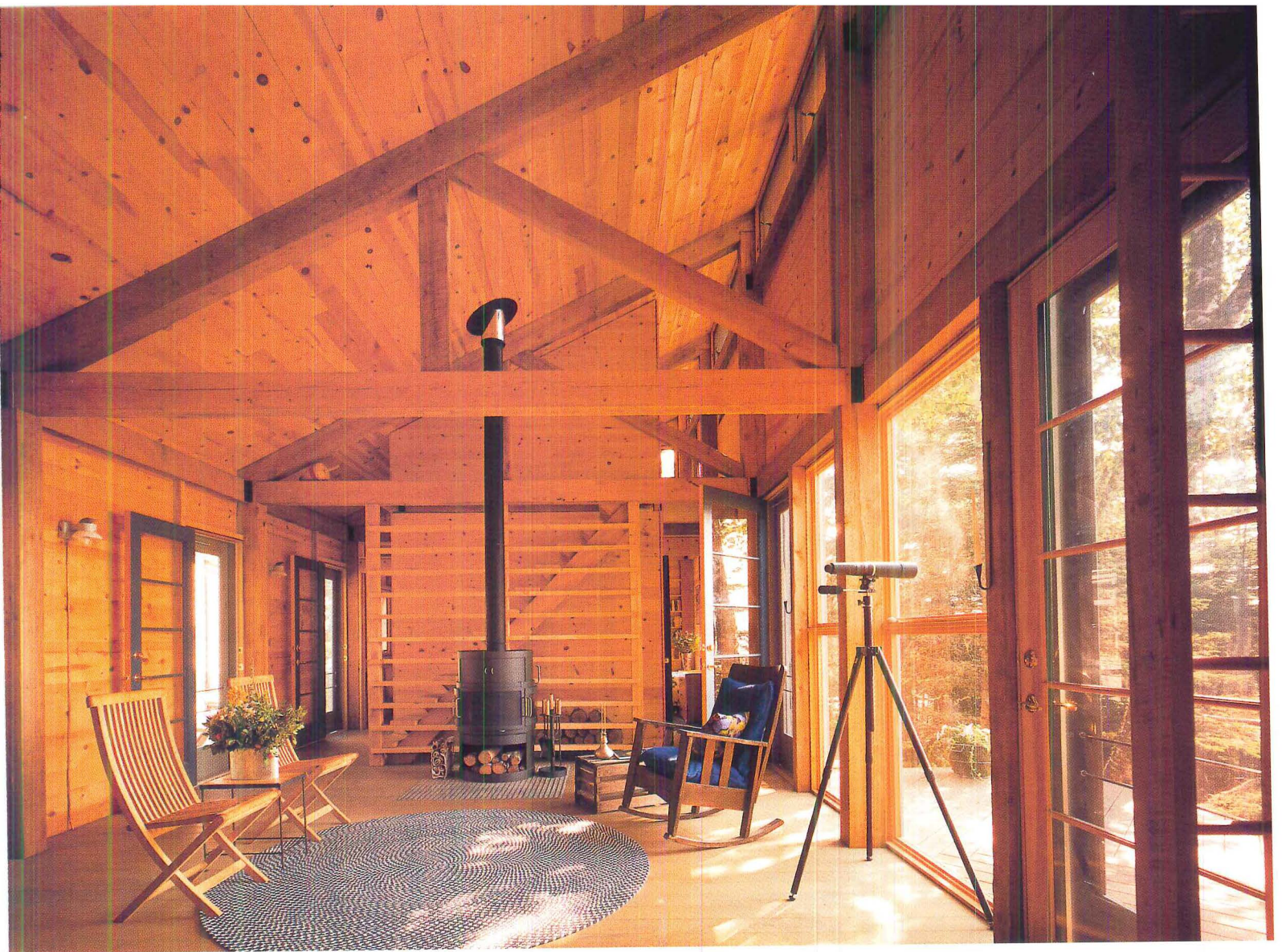
The living room's huge picture windows (above) take in every possible square inch of the island's exceptional views. Clerestory windows (right) allow light to graze the living-room ceiling in late afternoon. Laminated-wood decking, used as sheathing, doubles as the interior wall finish in the guest cabin (far right) and elsewhere.
