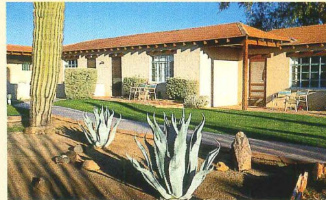
Stucco-clad Arizona resort structures are landscaped with naturally fire-resistant desert succulents to minimize the potential fuel supply that spreads wildfires.
