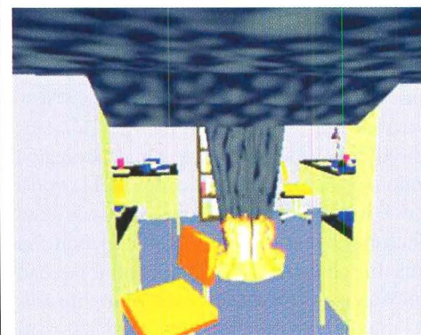
Researchers at NIST and the University of California at Berkeley are developing a fire simulation software system that creates a virtual walkthrough of a building during a fire, and displays a smoke-distribution model on screen.
