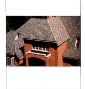
CertainTeed's Grand Manor Shangle® is a super heavy-weight shingle built on two full-size one-piece shingles with random 8" tabs applied on top. Patented shadow lines and a unique color palette give Grand Manor the look and depth of natural slate and wood. UL Class A. 40-year limited, transferable warranty on commercial applications. Algae-resistant. Meets ASTM D 3462—Tear Strength.
