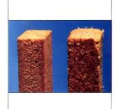
Duraflake MR moisture-resistant particleboard absorbs less moisture & exhibits minimal thickness swell compared to standard particleboard. For interior applications where exposure to high humidity & intermittent contact with water is common. It has a fine surface for laminating & exceptional strength. Applications include bathroom & kitchen cabinets & counters, casework, display fixtures, entryways & other moisture-prone areas. To request information call 1-800-887-0748 ext. 300.
