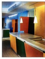
Fin Color Ply is a presurfaced multi-purpose plywood used for interior panels, furniture & cabinetry. Constructed with all Finland birch hardwood veneers, presurfaced on both sides with a durable colored translucent finish allowing visibility of the natural wood grain. Available in clear transparent, yellow, light brown, red, green, dark brown & opaque black. Panel size: 96" x 48"; Thicknesses: 1/2" (9-Ply) & 3/4" (14-Ply). Tel (310) 396-9991 Fax (310) 396-4482.
