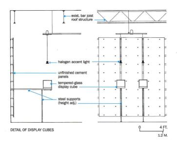
Steel tubes and bars support custom-made, tempered-glass cubes for displaying jewelry
