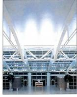
This revolutionary ceiling system offers nominal 12" (300mm) wide panels in lengths up to 19' 0" creating a clean, sophisticated, monolithic ceiling plane. Long spans are available with a soft beveled edge or a reveal edge. The system provides both acoustics and aesthetics with easily installed panels. Available in 8 finishes and 2 perforation patterns. For further information call 800-366-4327.
