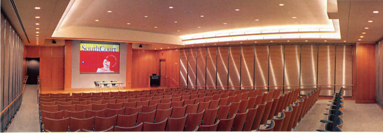
Woven stainless-steel mesh panels, a recurring motif throughout the South Court, define the back wall of the auditorium (above and opposite, top). Inside the auditorium, acoustical panels behind the mesh echo the warm color scheme of beech walls and seat backs. On the addition's third floor, a comfortable staff lounge offers veiled views of the original courtyard facade through glass walls (center right). Translucent glass encloses one of two interactive high-tech classrooms on the main level (below right).
