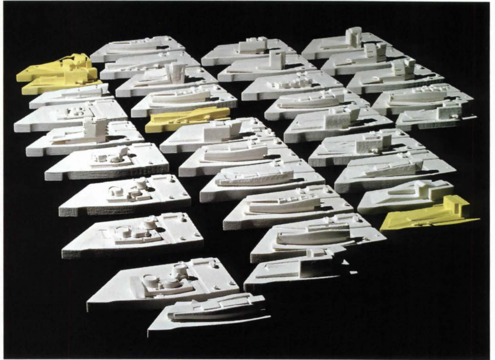
Rapid prototyping allowed the designers at Morphosis to quickly produce dozens of schematic massing models for a courthouse, which could be easily plugged in to a site model for closer examination.
