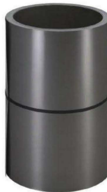
Zinc metal is produced into rolls with an initial shiny bright appearance.
