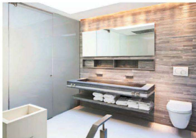
VANISHING ACT With the touch of a button, a low-level electric current runs between the panes of glass in the master bathroom to transform the walls from transparent (above) to opaque (right), allowing light in while retaining privacy.
