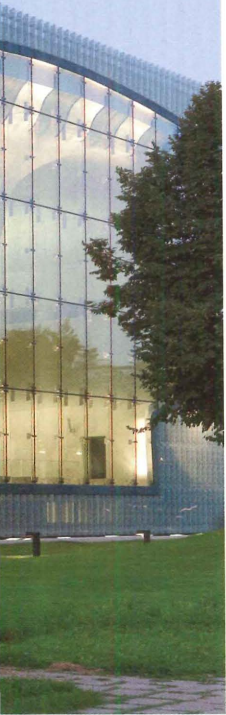
GRAND HISTORY The boxy museum, which is clad in angled fritted-glass panels separated by strips of perforated copper (above), conceals a cavernous entrance hall with curving concrete walls and a travertine floor (right).
