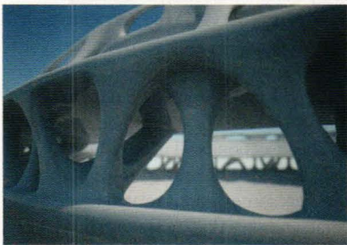
A completed 3D printed model can show the form and mass of a building or focus on a portion with as much detail as needed for design review.
