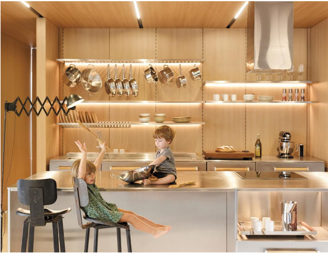
CHILD'S PLAY Channels in the kitchen's veneered backsplash (above) hold mounting brackets for easily reconfiguring shelves and racks. The kitchen is designed as freestanding modules (right) to be moved when residents do.
