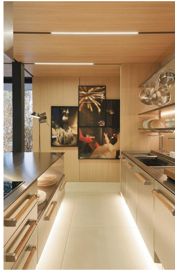
CHILD'S PLAY Channels in the kitchen's veneered backsplash (above) hold mounting brackets for easily reconfiguring shelves and racks. The kitchen is designed as freestanding modules (right) to be moved when residents do.
