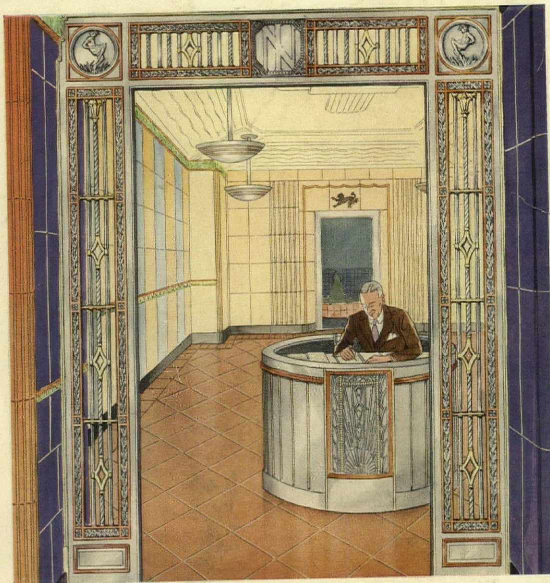
● View of the Terra Costa Room, Procurement Division, Washington, D. C. Striking harmony of color is obtained by the use of Nickel Alloys, yellow brass and red brass in the construction of the trellis grille and information desk.
